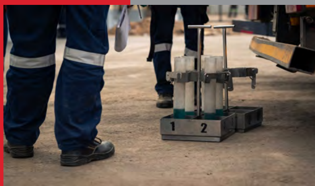
Sampling of marked fuel for verification at a retail site in Mozambique
